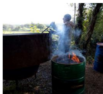
The stages of producing Biochar. 1. Gathering brush. 2. Loading the kiln. 3. Packing the still burning materials into barrels. 4. The end result. Photos: 1&2. Edmund Gabriel. 3. Judith Tranter. 4. Biochar Wales
