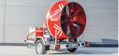
A purpose-built, special designed one-axle trailer. Compact and light-weight for extreme handiness. One person can easily position the MGV<sup>®</sup> with the big handles on both sides.
