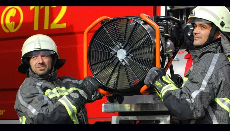
High performance fans allow effective ventilation of burning buildings and sites of operation from smoke, heat and toxic gases. The conditions for the fire fighters are significantly improved. The attack group can orient itself faster inside the object and fight the fire more effectively.
