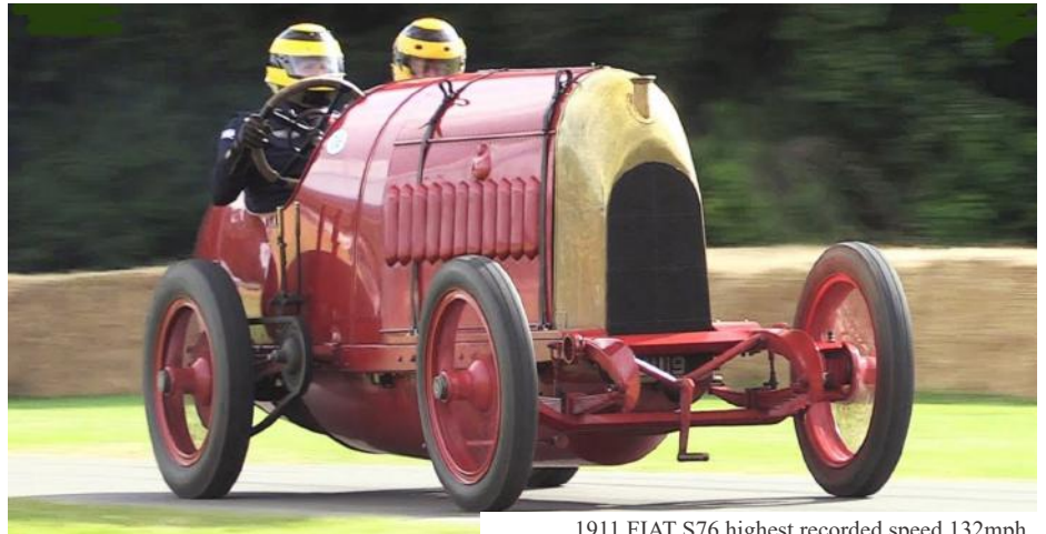
1911 FIAT S76 highest recorded speed 132mph. Videos available on YouTube, including starting it up.
