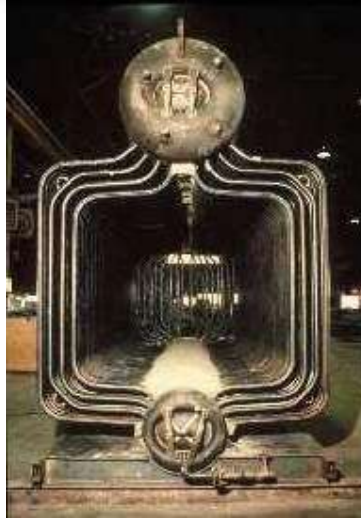
Watertube Boiler "O"
