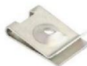
20649 Screw Size: M3.5 (#6) Panel Range: .5mm - 1.5mm Center of Hole to Edge: 8mm
