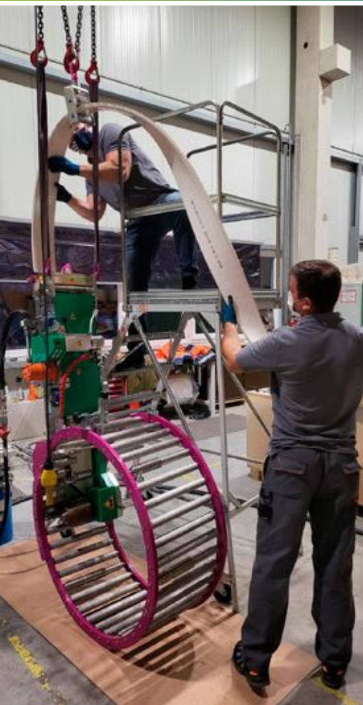
The SWP winding cage and drive unit being prepared for deployment to the site
