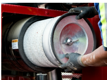
Donaldson Air Cleaner with Safety Element (Standard)
