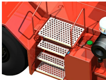
Easily Replaceable Bolted Steps & Handrails
