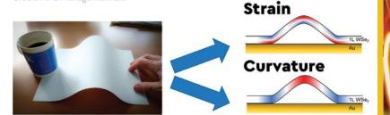
Schematic diagram illustrating the distinction between strain and curvature in wrinkled material.
