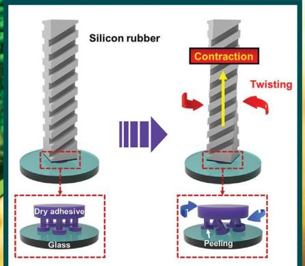
The robotic device has a vertical silicon rubber (left) with dry adhesive separated into several triangular pads. The pads stick to the glass as they are pressed down and peel off with upward twisting motion (right).
