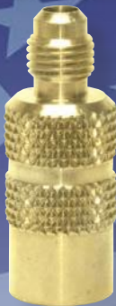
92863 R-410A Mini-Split Adaptor 5/16" (1/2"-20) Female w/Adjustable Depressor x 1/4" Male w/Valve Core
