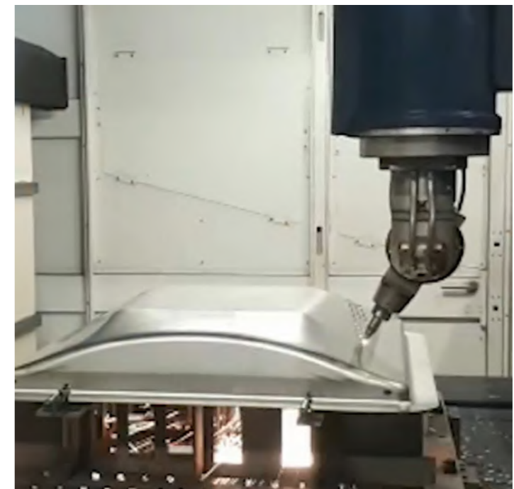
Cutting off excess material
