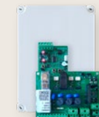
cod. 79220022 Meteor plus teleinvertitore trifase three-phase control unit
