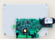
cod. 79240002 AcruX plus inverter monofase single-phase control unit
