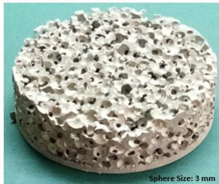
Metal foam Heat Exchangers of various pores size: An aluminium foam heat sink
