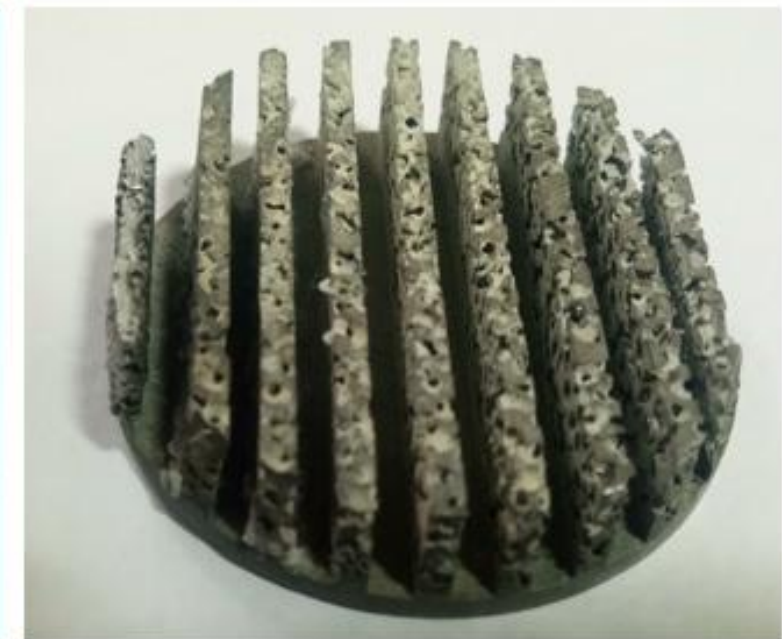
Metal foam Heat Exchangers of various pores size: An aluminium foam heat sink
