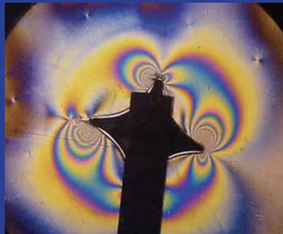
Kaleidoscopic vision: Scattered fringes as seen in the polariscope designed by Prof Srinath
