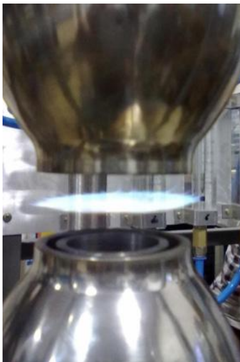
Counterflow Flame: Canonical flame to study and evaluate combustion chemistry and emission formation
