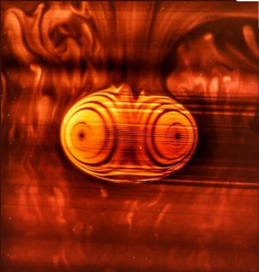
Solar thermal energy storage: Laser induced flow visualization imaging of thermal energy storage systems
