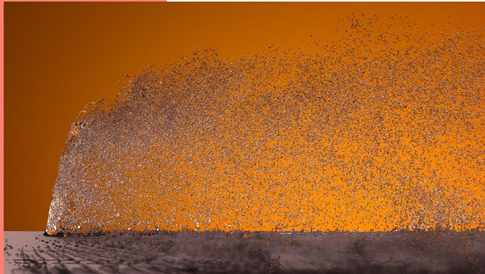
Simulations of liquid jet breakup in crossflow
