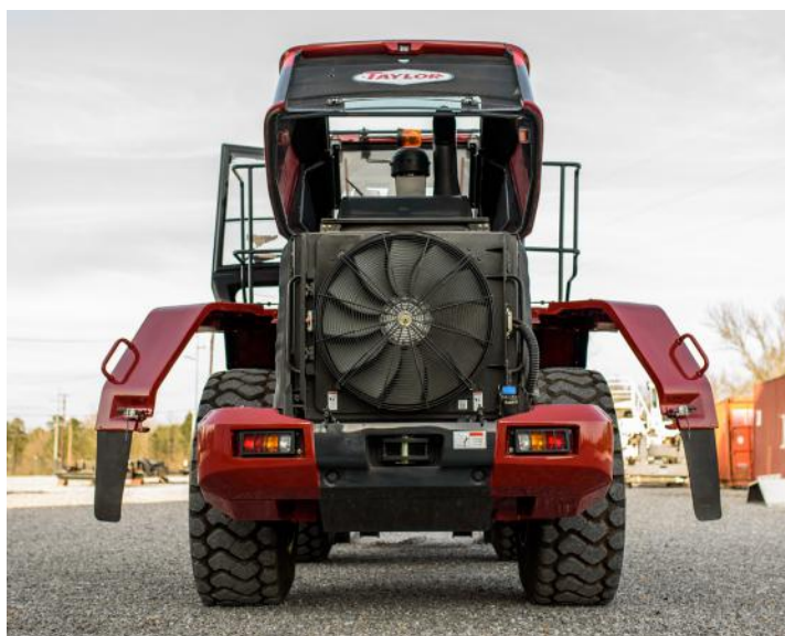
The rear full fenders swing out for easy access to the engine compartment. The electrically actuated, wide opening fiberglass hood of the Taylor T-1045 gives you easy access to the engine and its easy-to-reach service points. The radiator also swings out for ease of service.
