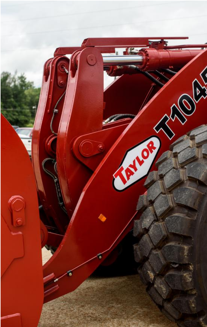
The Taylor T-1045 has been designed to offer optimized visibility. A panoramic view cab with curved front glass has been paired with well-positioned lift arms to allow the operator a clear line of sight to the attachment at ground level.
