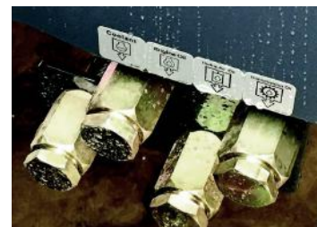
Autolube is a standard feature on the Taylor T-1045. All pressure taps and site gauges are easily accessible. Fluid drains provide environmentally friendly drainage capability and are grouped together for convenient serviceability.
