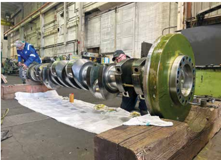
Reconditioning the spare crankshaft at United Engineering.
