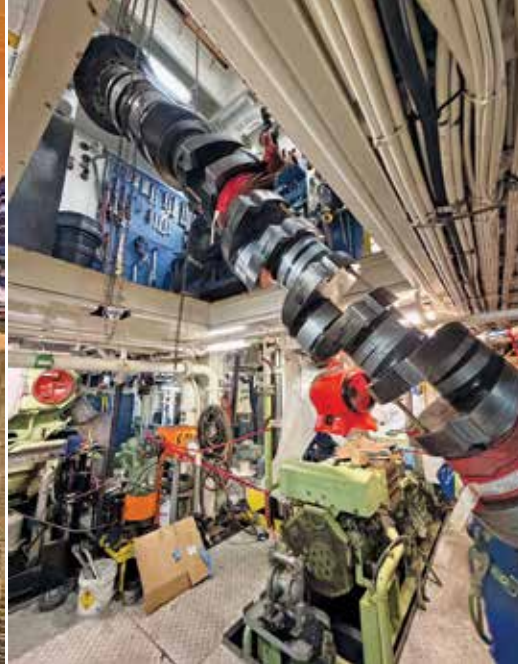
The reconditioned crankshaft being returned to the engine room.
