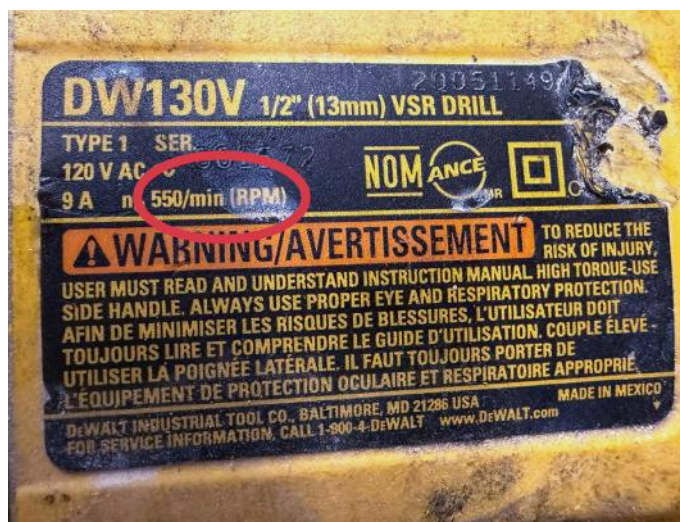
Check the RPM rating on your drill and match that to the mixing speed you need.
