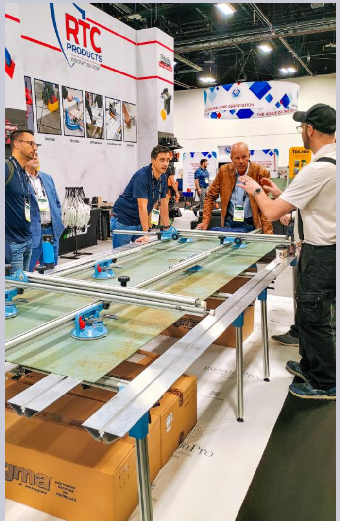
The Sigma Work Table was designed for working with thin panels but is easily modified for all tile projects.
