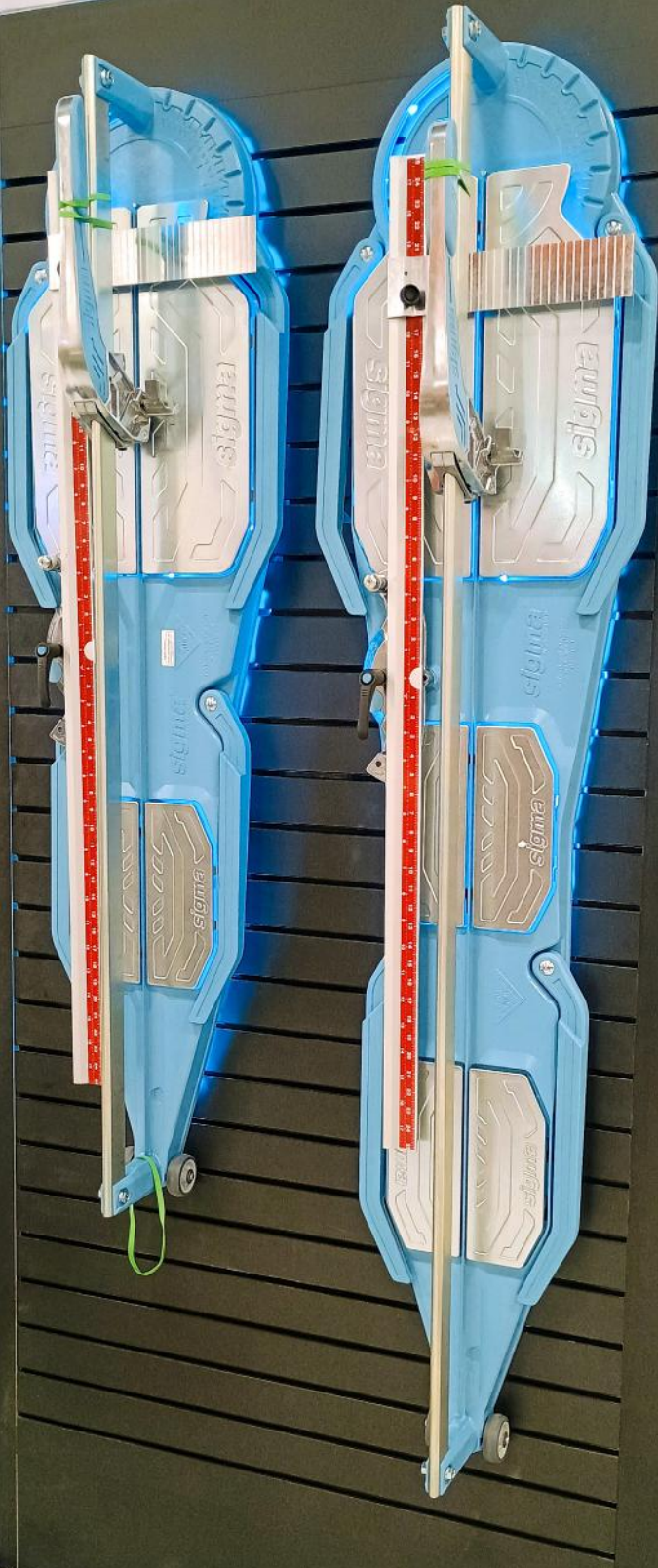
The Sigma Series 4 NEX push-handle tile cutters feature a robust design built to handle rough and large tiles up to 3/4" thick.
