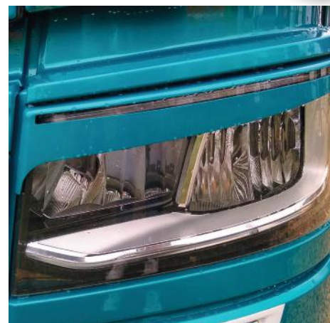
Part No. 20000073 EYELIDS SCANIA NEXTGEN TYPE 3 Set of 2pc, with cutout for indicator light. Mounting with double sided tape. € 85,00 excl. VAT / € 102,85 incl. VAT
