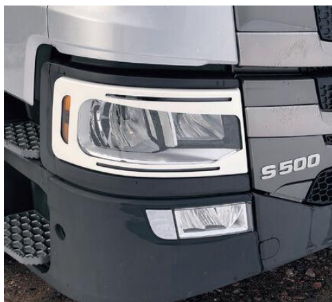
Part No. 20000073 EYELIDS SCANIA NEXTGEN TYPE 3 Set of 2pc, with cutout for indicator light. Mounting with double sided tape. € 85,00 excl. VAT / € 102,85 incl. VAT
