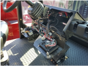
Flip-down Dash with Color/Number Coded Wiring (Standard)
