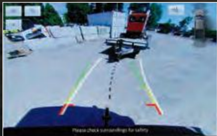
REAR VIEW CAMERA WITH DYNAMIC HITCH ASSIST Standard on all trim levels, it helps you hook up your trailer with ease.
