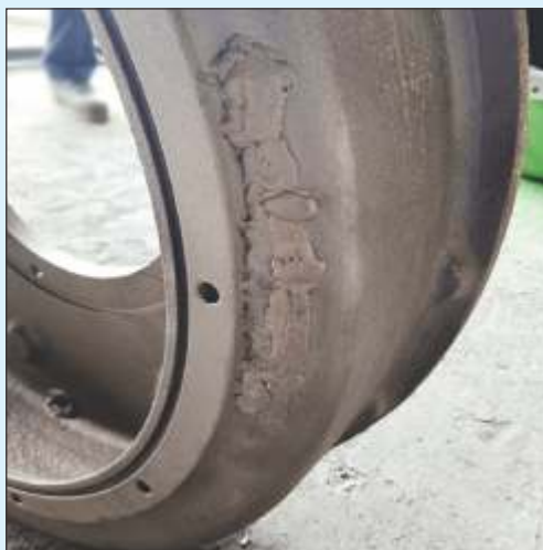
The steam cooker's top cover had suffered from high-temperature corrosion, with constant exposure to steam at 130°C.
