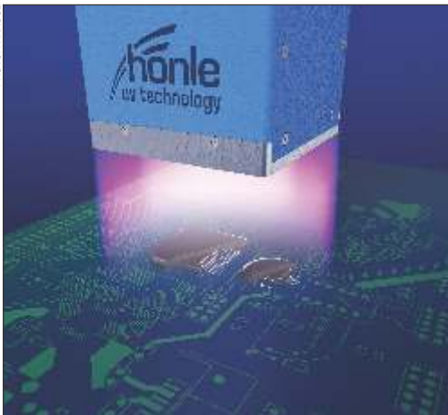
Black epoxies being cured with UV LED light.
