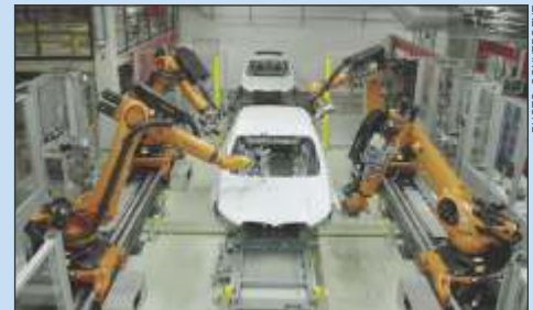
'Automappps' supports various sensors for paint inspection – robot-guided and stationary. Various robot manufacturers, tools for sanding and polishing and adapters are also supported.
