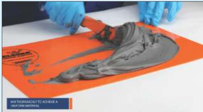
Belzona 1511 mixed at a metric ratio of five parts base to one part solidifier, achieving a uniform streak-free grey color.
