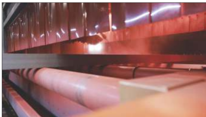
At the entrance to the automatic paint system special sensors measure the dimensions of the work pieces – down to the last mm.
