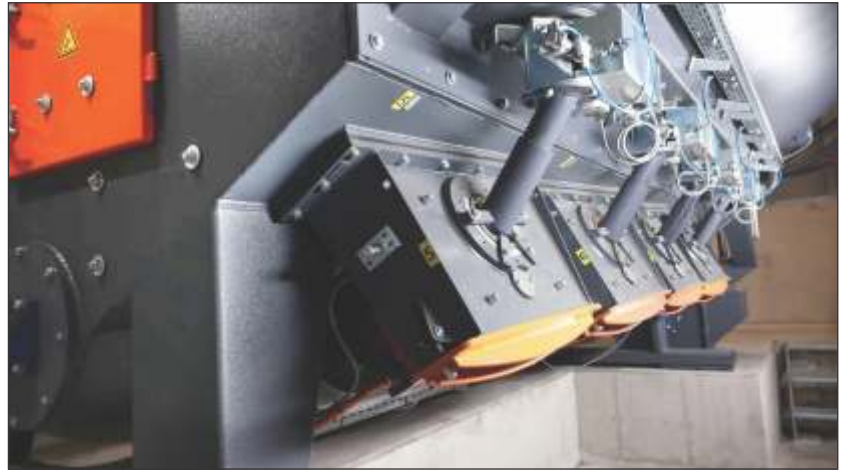
The eight Gamma 400G high-performance turbines with “Y” shaped throwing blade guarantee consistent high-quality shot blasting results.
