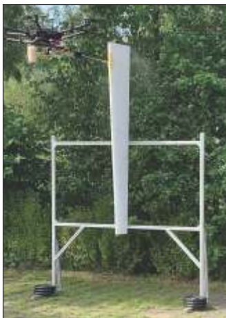
Coating drone during a spray test: The coating material is applied by the drone via a lance.
