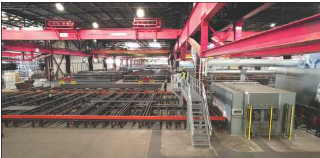
The preservation line with shot blast machine and automatic paint system can handle work pieces weighing up to 12 tons. The design was adapted to the existing building containing an overhead crane.
