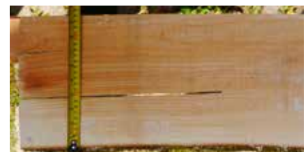
Figure 8: Sawcut in the fresh-dried sycamore, showing no tendency to close or open
