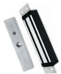
Aluminium-zinc, mortise-mount, fail-safe, 270kg holding force, 12V/24VDC
