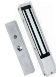
Aluminium-zinc, surface-mount, fail-safe, 270kg holding force, 12V/24VDC
