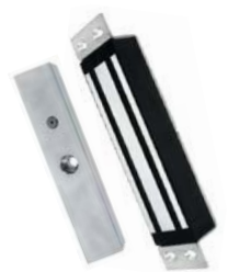
Aluminium-zinc, mortise-mount, fail-safe, 270kg holding force, 12V/24VDC
