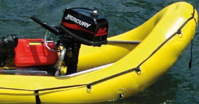
MAIN PIC: Oceanid RDC. Invented in 1996 in Washington State in response to a request for a specialist ice-rescue craft, the Oceanid RDC has lately spawned many copies. This image shows the optional transom for mounting an outboard which a number of larger sleds/rafts also offer.
