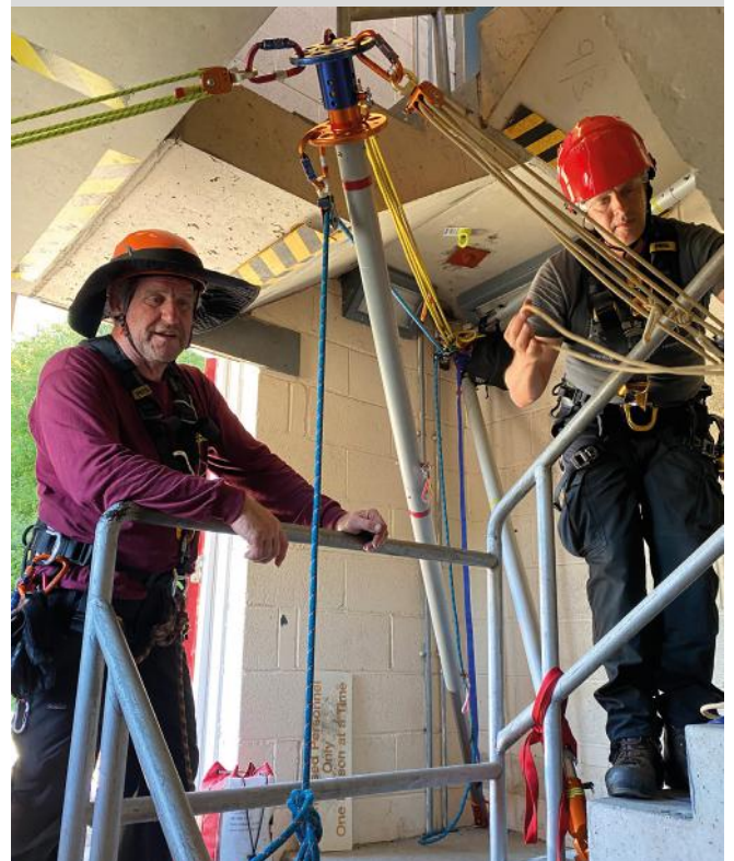
BELOW: Delta guyed gin pole using three AZTEK at 120° angles. Photo from Llangollen, Wales, AHDW workshop with R3 Safety & Rescue in 2022.
