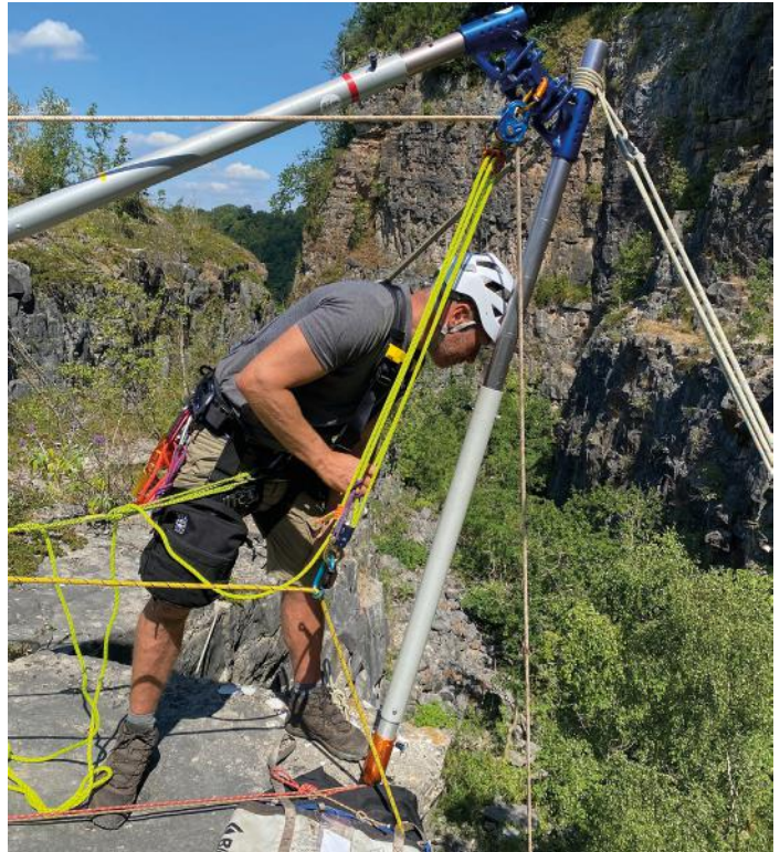
ABOVE: An edgeman working under an Arizona Vortex SA-Frame using both ends of the AZTEK. The personal side is used to restrict travel with a Purcell prusik to the rear/left to protect him from falling off the edge. The other end (system side) is being used with SOF to temporarily elevate the slack belly line during the edge transition. Photo from Bristol, UK TSRW workshop in 2022.
