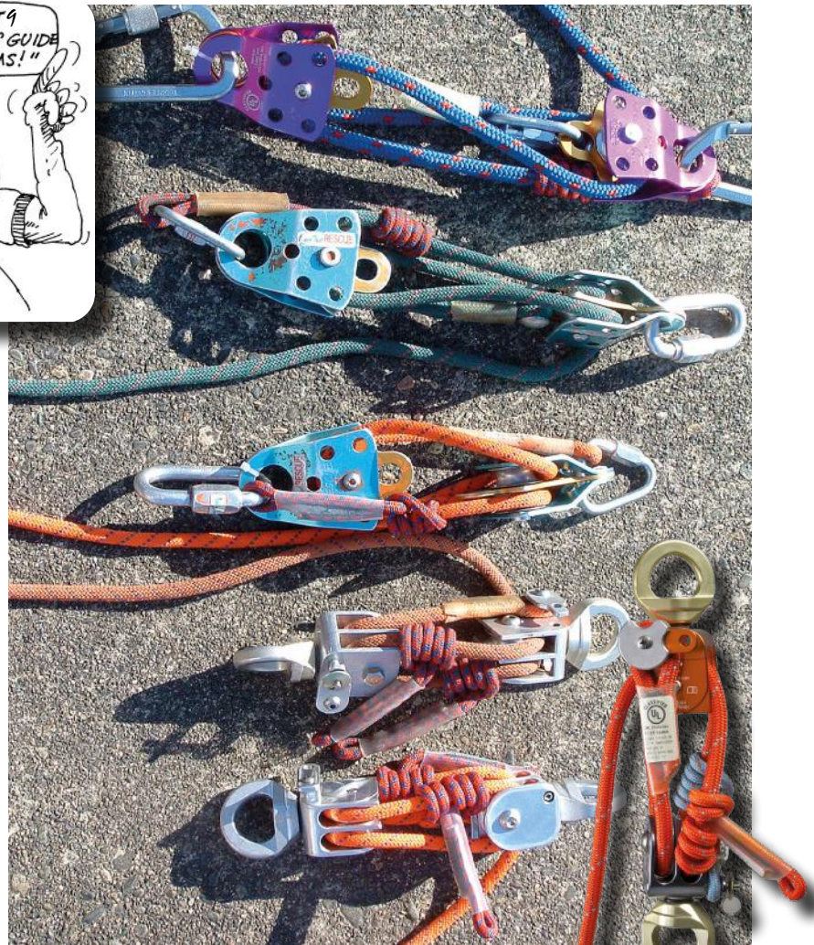
ABOVE: The slow evolution of the AZTEK which we called the "set of fours". The small jigger pulley system kept getting smaller and smaller so that it became a very compact unit. It started with the original double pulleys from Rock Exotica (blue) then Petzl made the Gemini (purple-top system). The first milled version was made by Rock Thompson but was slightly too large for our liking. The final non-anodized version is on the bottom and became the final production model as per the CMC version (inset above).
