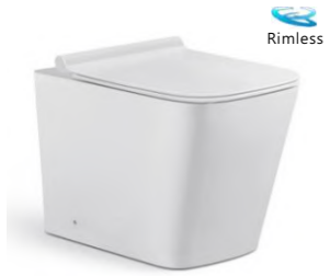
W 2051B Washdown floor mounted toilet Size:590x350x410mm P-trap:180mm
