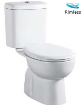
W8008 Washdown two-piece toilet Size: 680x360x780mm P-trap: 180mm S-trap: 225mm
