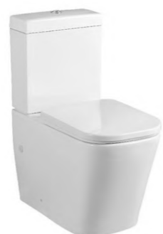
W6014 Washdown two-piece toilet Size: 670x370x795mm P-trap: 180mm S-trap: 150/250mm
