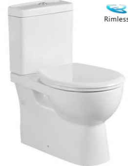
W8011 Washdown two-piece toilet Size: 620x355x760mm P-trap: 180mm S-trap: 150/220mm
