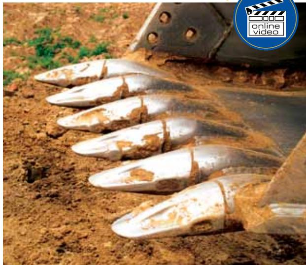
Komatsu's KMAX tooth system offers durability in more than 20 tooth styles for a wide range of excavators and wheel loaders. It's easy and safe because the system requires only a socket wrench — no pins to hammer — to remove and replace teeth from the adaptors.
