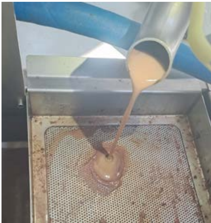
Figure 1 Greasy effluent at one of the food processing facilities partaking in the study by the ARC
