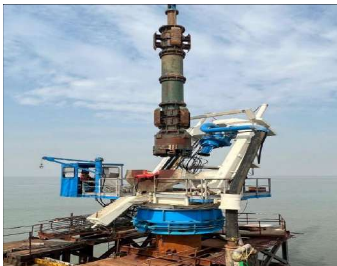
Figure 5: Drilling Setup and BHA Installation in RCD
