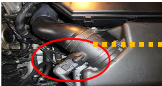
AIR FLOW SENSOR
