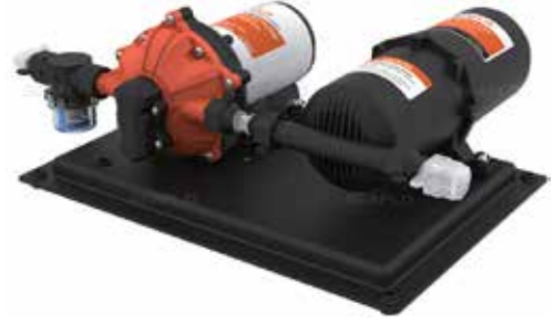
SR09684 Seaflo Tanklı Hidrofor 12 V - 20.8 lt. / dk SR09686 Seaflo Tanklı Hidrofor 24 V - 20.8 lt. / dk Tank: 1 Lt , 60 Psi, 37x35 cm, Çıkış: 13 mm
