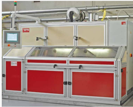
Burst test stand capable of performing burst tests on hose assemblies up to 10.000 (145000 psi)
