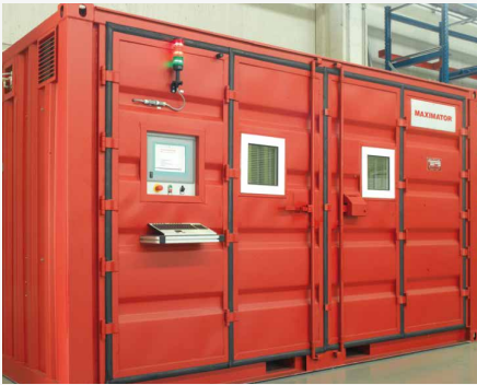
Proof pressure test stand able to pressurize hose assemblies up to 6.000 bar (87000 psi)
