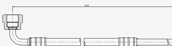
Elbow Female 90° 3/8 + Copper brazing tube
