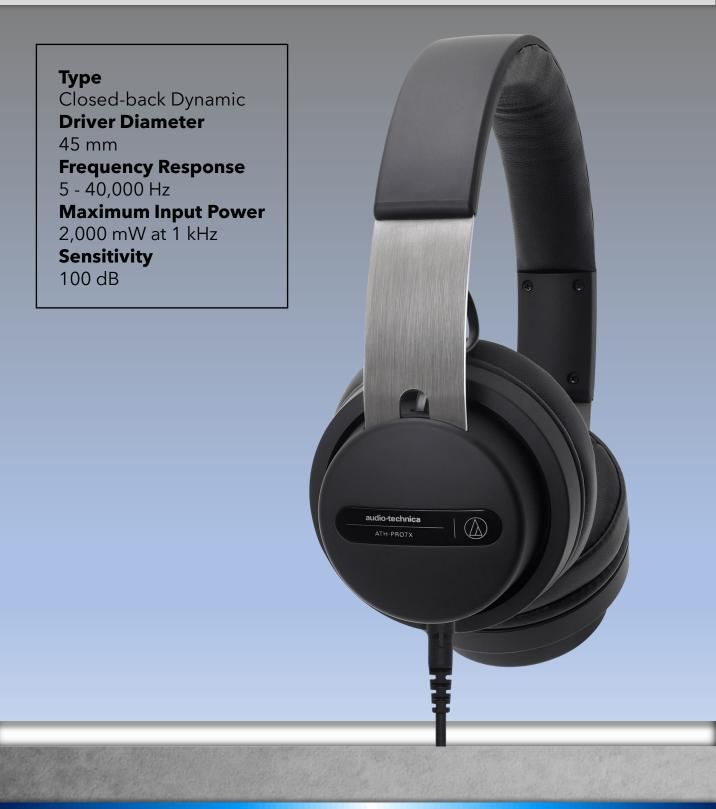
The ATH-PRO7X professional DJ headphones combine the comfort and low-profile style of an on-ear design with powerful 45 mm drivers capable of handling 2,000 mW of input power. This combination gives DJs extremely accurate high-fidelity audio reproduction – even at loud volumes – from a pair of headphones that are easy to wear through even the longest gigs.
