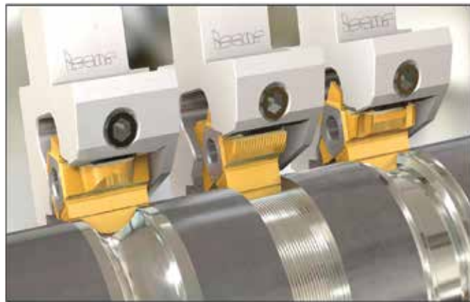
Fig. 4 - PENTACUT-27 starlike blank inserts enable fast customized solutions for complex profile grooving.
