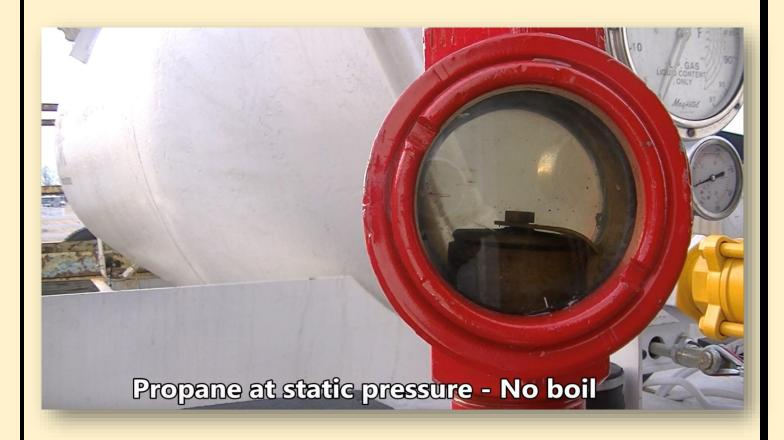
vapor pressure in the container is equal to the pressure of the surrounding atmosphere. In a closed container, boiling (vaporization) will stop when this equalization is achieved.
