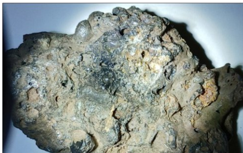
Slag with outgassing vents
