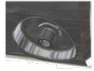
Connector in underside of Load Cell head
