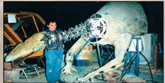
Robotic Dinosaur - Internal workings of neck
