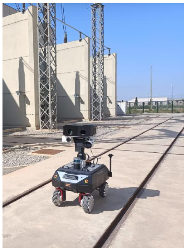
Robotnik robot with OFIL UV camera, deployed by BCB for substation inspection
