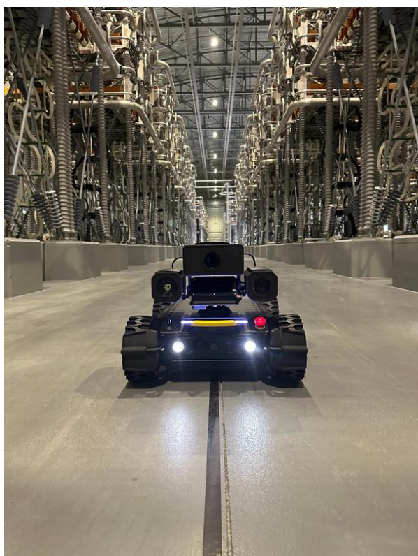
OFIL UV camera integrated on Ross Robotics autonomous platform for HVDC hall inspection
