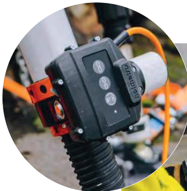
Holmatro remote controller and multi-strut load sensor.
