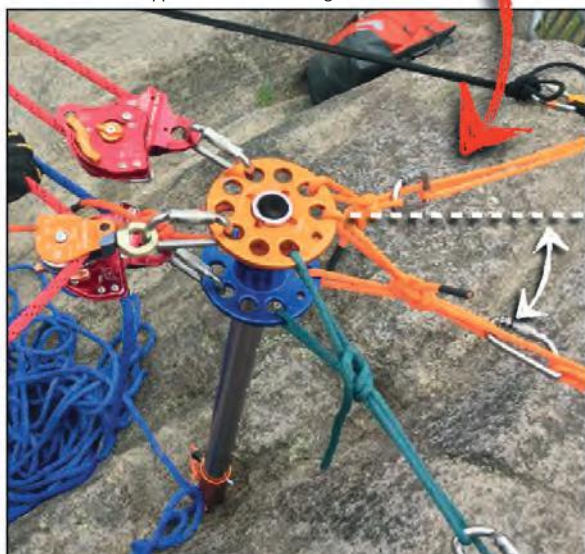
A "Bombproof" focused floating anchor with three back ties and one opposition front tie using an AZORP®
