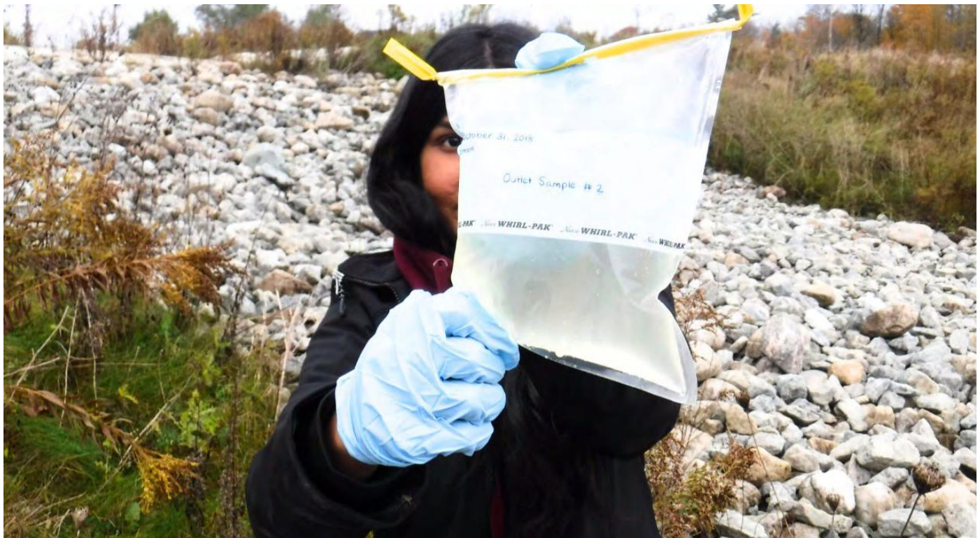
Crozier's Amanda Pinto, P.Eng., MEL, collects water samples from an outlet of a stormwater management facility.
