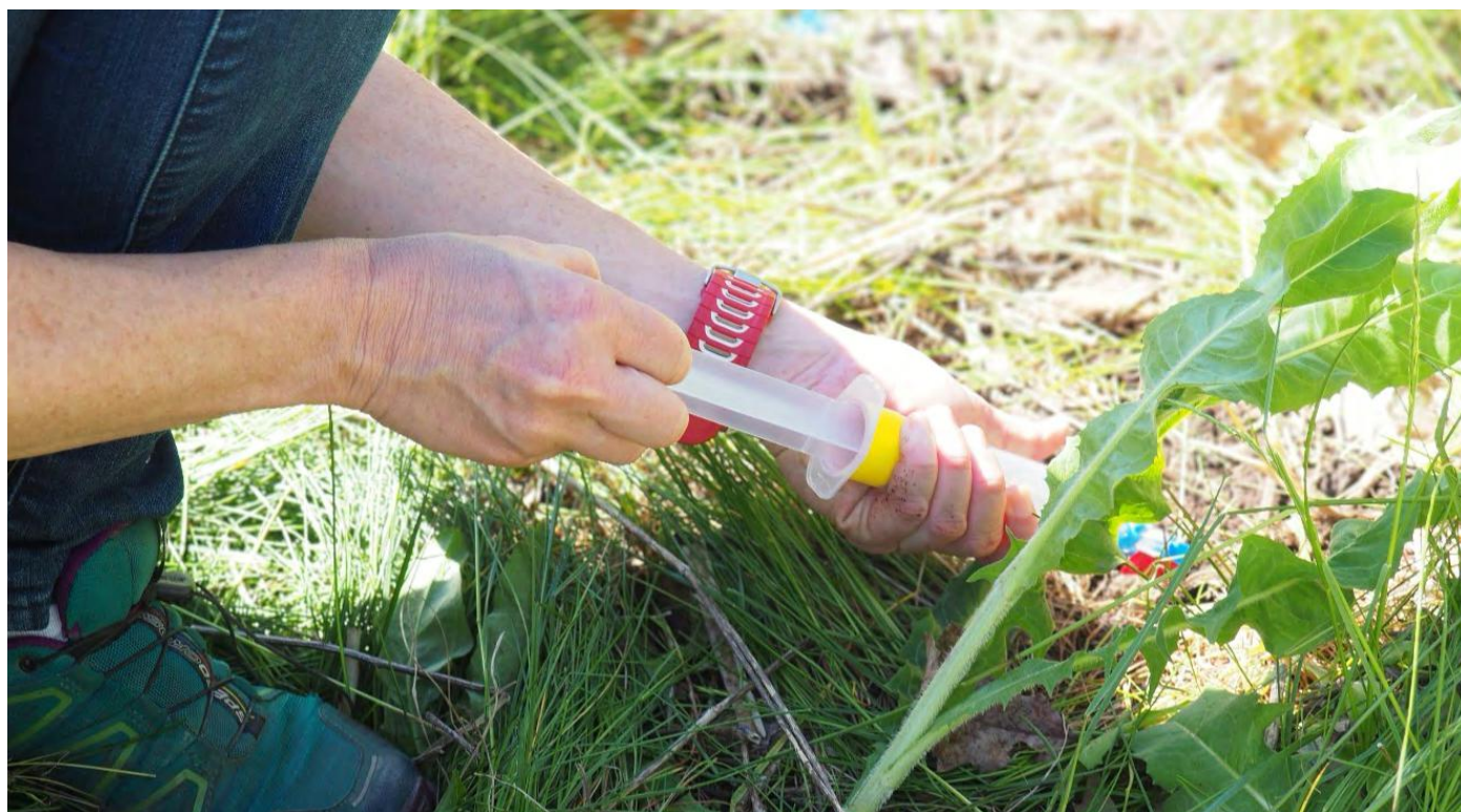
A researcher uses specifically designed devices to extract stormwater samples from varying depths of soil media in bioretention systems.
