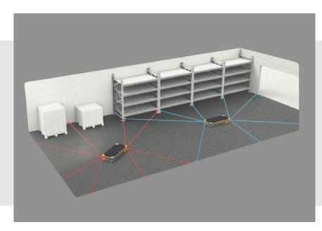
The Move utilizes natural navigation through safety scanners positioned at ground level. By referencing structures and contours in the environment, it determines its location without the need for complex infrastructure such as inductive wires, magnets, or reflectors. Simple reflectors can be incorporated where needed, providing flexibility in setup.
