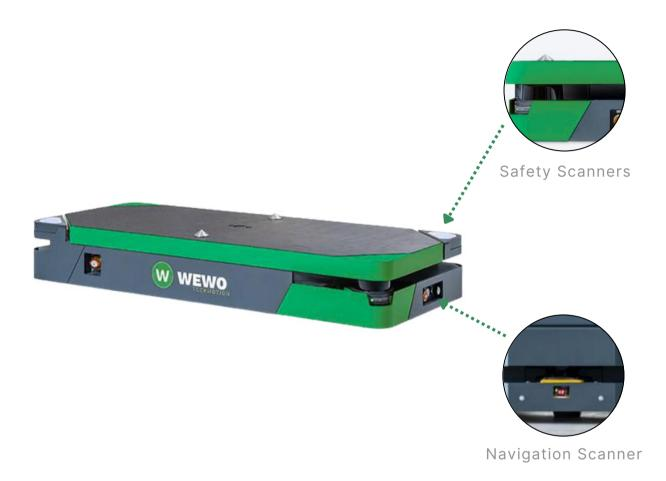
The AGVs are equipped with advanced safety systems designed to protect employees, infrastructure, and the robots themselves.
