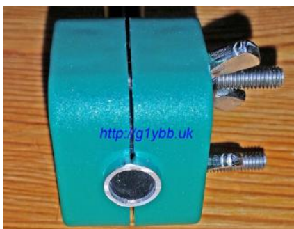
Using Clamps to mark Centreline
