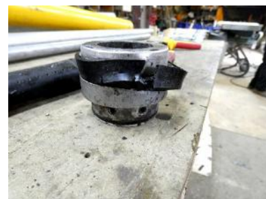
Damaged seal from wrong lubricant
