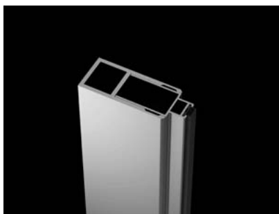
Eos – Profile + 2 cm (except from Eos DWJ II). You should replace standard magnet-catch U profile with the extension profile P01-137195001.
