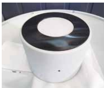
Hidden inside: a puck, the centrepiece of a SIP® bearing. The photo was taken during the overhaul of a prototype bearing following testing. Photo: MAURER
