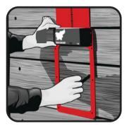
Using a marker, trace the inside edge to create a drilling guide.
