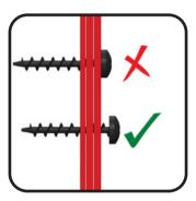
The door will not work if screws are overtightened. Please ensure yours matches the diagram.
