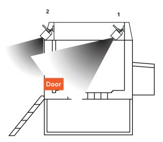
(2) Exterior Camera: Your exterior camera should have a clean view of your coop perimeter in close proximity. Ideally, the outside of your Automatic Door is visible in the camera frame, as well. We recommend placing within 6-9 feet of perimeter for the most accurate image and sound recognition.
