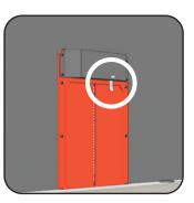
Simply pull the plastic tab from the black battery compartment. This will activate FACTORY SETTINGS MODE. Your door is now programmed to automatically open at sunrise and close 20 minutes after sunset. **That's it!**
