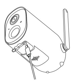
Easily charge your CoopCams with a micro-USB cable. Fully charge the camera batteries during the day to prevent interruptions to nighttime surveillance. Charging can take up to 14 hours depending on how depleted they are.
