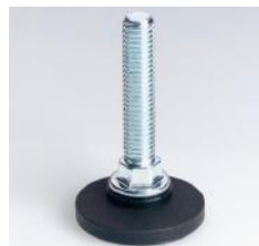
REF: AM-FOT005 30MM DIA. FOOT M10X35MM, INTEGRAL NUT HEIGHT ADJUST 25 MM LOAD RATING 1000 KG
