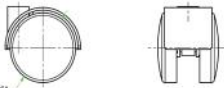
REF: AM-CST010 CASTOR - 2" BLACK PLASTIC UNBRAKED DIAMETER 50.0 MM / 1.969" LOAD CAPACITY 60KG COLOUR BLACK
