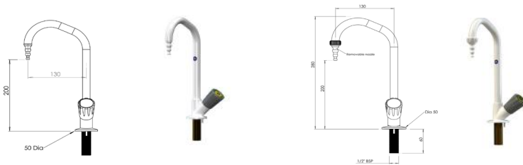
Ref: AM-900103 Fixed Swan Neck With Fixed Nozzle AM-900101 Thread: 1/2 " BSP Cold (AM-900103) Hot (AM-900101)
