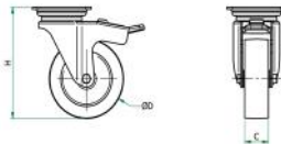
REF: AM-CST002 CASTOR-2" SCREW IN RUBBER CASTOR - GREY BRAKED DIAMETER 50.0 MM / 1.969" WHEEL WIDTH 18 MM LOAD CAPACITY 40KG COLOUR BLACK
