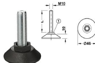
REF: AM-FOT008 FOOT SCREW-ADJUSTABLE SCREW-M10 THREAD WITH FIXED FOOT LOAD RATING 1000 KG
