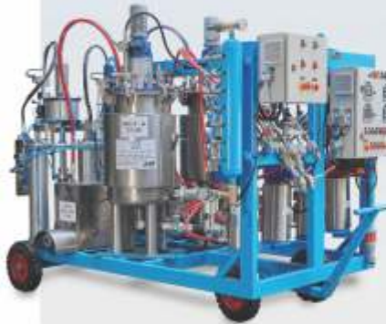
PFP / INTUMESCENT COATING SYSTEM
