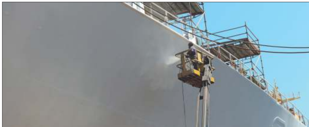
Ships and offshore platforms need coatings that resist saltwater, biofouling, and UV exposure.
