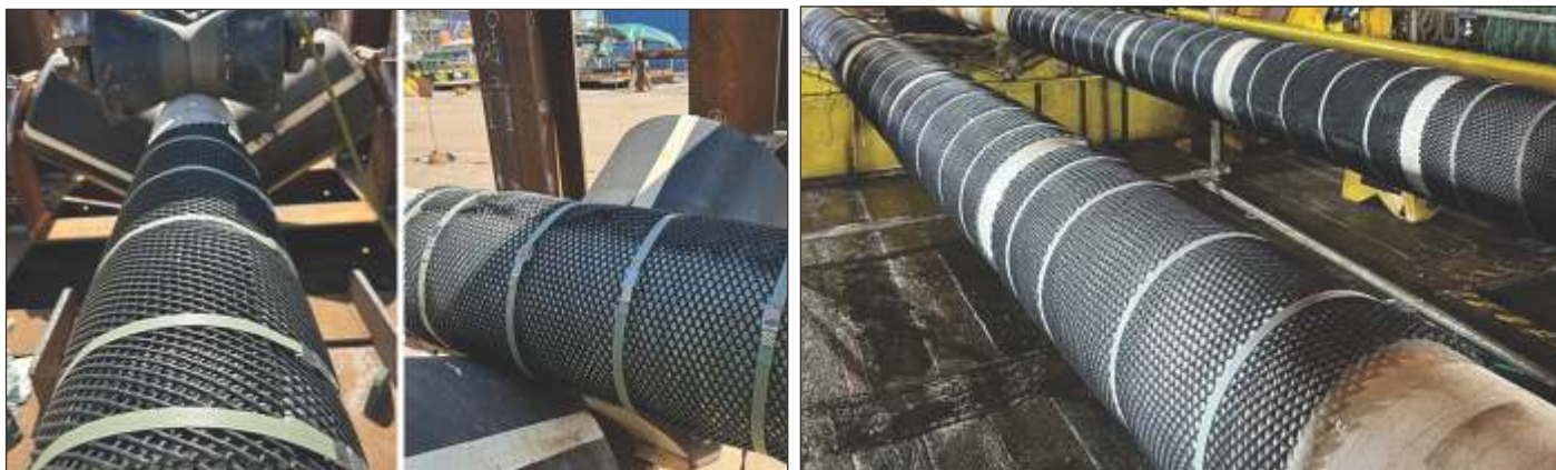
(Top row) Roller box test simulating the pipelay vessel's stinger operation, and further testing during the Pre-Production Test (PPT) stage.
