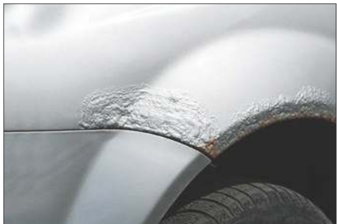
Vehicles stored in open yards for even a few days may begin to show signs of corrosion.
