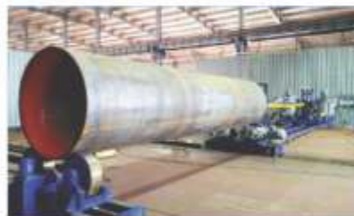
Internal Automatic Pipe Coating
