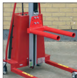
Double Spindle - EP06 ø 50 x 500mm (260mm centres) Capacity: 250kg £195.00
