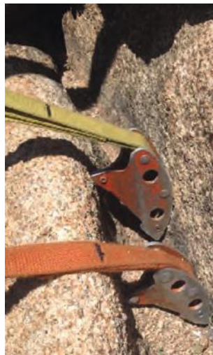
Above: Artificial anchors showing two pieces of rock called “Tricams” both used in an active position.
