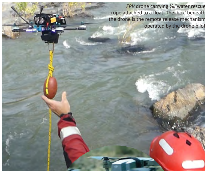
Initial testing of the pulling power of the FPV drone carrying 3/16" water rescue rope rather than carrier line and a REACH device
