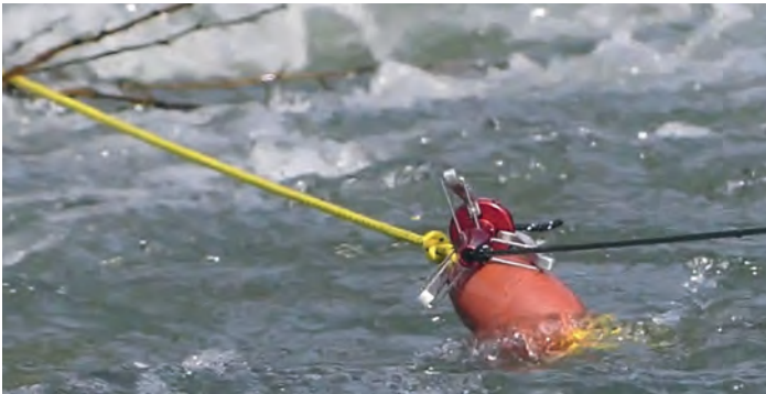
The REACH LCD is dropped by the drone across the floating rope and is then pulled in until it runs up against the float and the captured rope can then be hauled back to shore.
