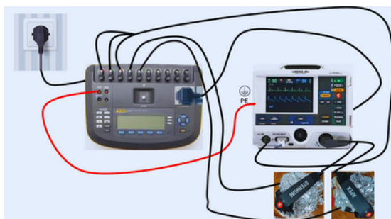
Figure 3 : Connection Between Medical Equipment and Analyzer
