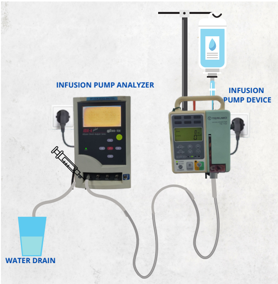
Figure 6: Connection Between Medical Equipment and Safety Analyzer
