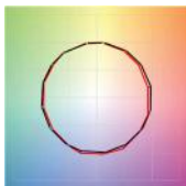
ERCO LED 3000K R_f 92 R_g 98 | R_a / CRI 92
